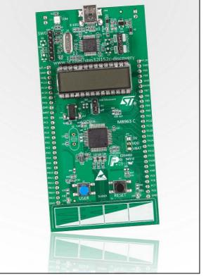
They are based on an STM32L152RBT6 and an STM32L152RCT6, respectively; and include an ST-LINK/V2 embedded debugging tool interface, an LCD (24 segments, 4 commons), LEDs, pushbuttons, a linear touch sensor or touchkeys.
